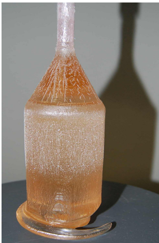
Figure 9. Crystal from Terbium Gallium Garnet with target diameter showing a sudden transition to spiral growth because it has the tendency to a larger diameter by flaring. Reproduced with permission. [3] Copyright 2016, Elsevier.
