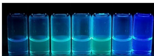
Figure 3. Demonstration of QY increase of compounds as 0.02 M DCM solution (left to right: 9j , 7j , 8d , 7i , 7c , 10h , 10b ).
