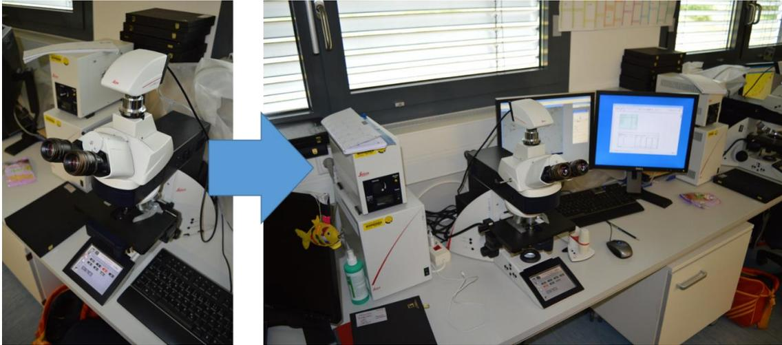
**Fig.6 Desktop workstation** featuring the Leica DM6000B® motorized microscope with digital interface
