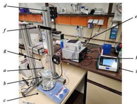
Fig. 2. Experimental setup of the thermoresistometer for controlled thermal exposure; a 50 µL capillary; b water bath; c hotplate stirrer; d solenoid; e timing relays; f capillary holder; g rocker arm; h cooling fan; i datalogger.
