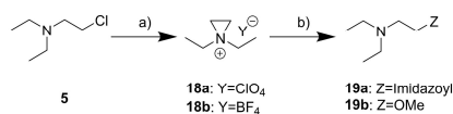
Scheme 3. Synthesis of the aziridinium ion of 2-chloroethyl diethylamine 5 and subsequent reaction with nucleophiles. a) AgClO 4 or AgBF 4 , dry Acetone; b) Imidazole or MeOH, dry CD 3 CN, RT or 50 °C.
