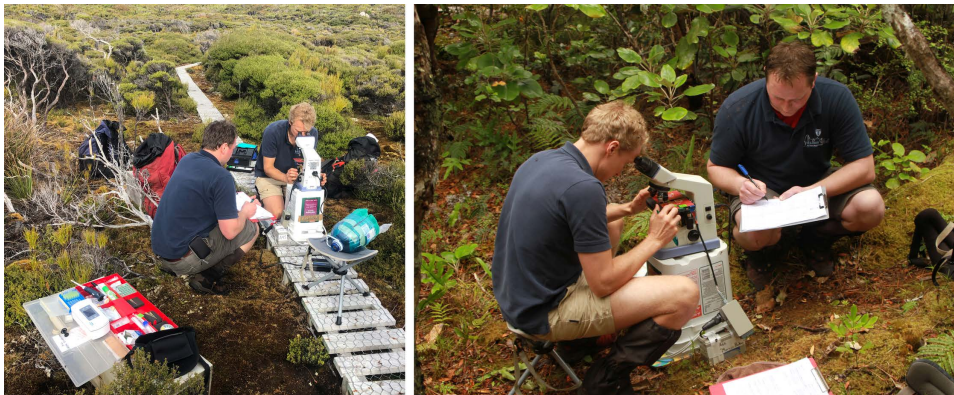
Fig 4. Semen analysis was performed immediately in the field using mobile equipment. This included a microscope with 40 X - 400 X magnification and phase contrast and a heating pad attached to a 12V mobile motorcycle battery. The individuals depicted in this manuscript have given written informed consent (as outlined in PLOS consent form) to publish this picture and these case details.
