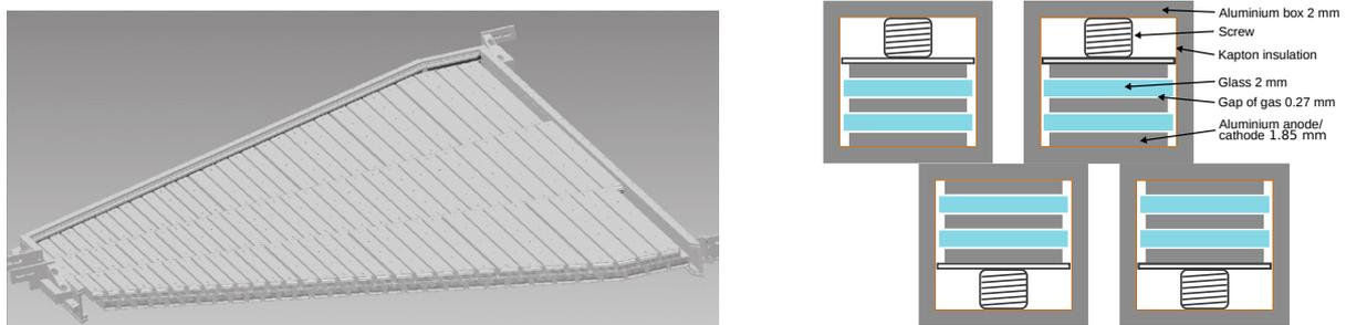
**Figure 4.3:** (left) Schematic drawing of a full HADES RPC sector [120]. (right) Schematic drawing of a single HADES RPC cell [119].
