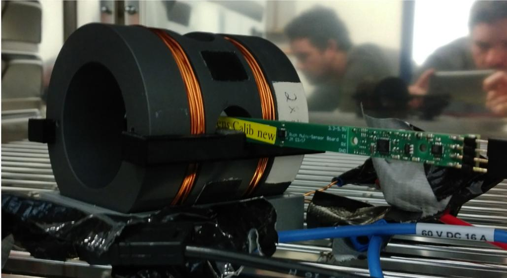
**Figure B.2:** Photography of the Helmholtz coil with a sensor board in measurement position inside the climate chamber.
