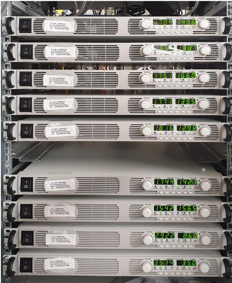
**Figure 5.16:** Low voltage power supply rack with running RICH FEE next to the detector. The voltages (left) and drawn currents (right) of each power supply are visible. All power supplies are connected to LAN and are accessible via EPICS.
