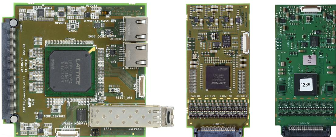
**Figure 3.28:** (left) The RICH combiner module with its central Lattice ECP3 FPGA, the SFP+ cage for the fiber connection to the upper readout stages and two RJ45 connection for Trigger and Clock distribution. (middle) A DiRICH version 1 with one central Lattice ECP5 FPGA and the 32 channel amplification stage near the SAMTEC connector. (right) A DiRICH version 4. It has two small Lattice MachXO3 FPGAs for threshold settings, an improved layout and easier FFC connection.
