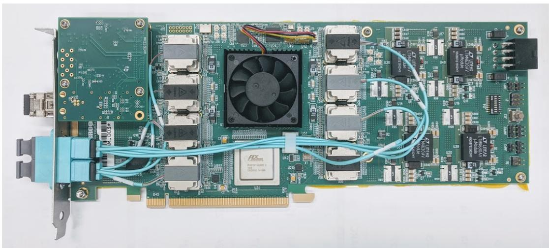
**Figure 7.1:** Photography of the FLX-712/BNL-712 readout card with timing mezzanine card [94]. It will act as the CRI board in the mCBM experiment and for the RICH also in the CBM experiment.
