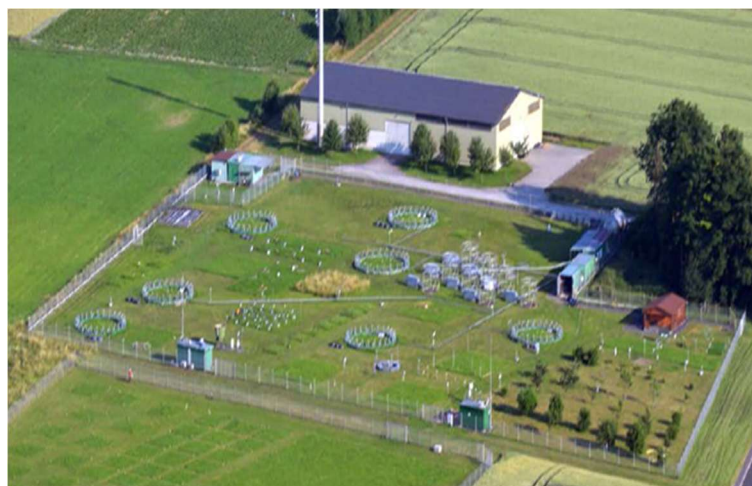
Figure 1 Giessen Free Air Carbon dioxide Enrichment (GiFACE) system of the „Environmental monitoring and climate impact research station in Linden“, near Giessen, Germany. Six rings of the GiFACE: three rings of control with ambient atmospheric CO 2 (aCO 2 ) and three rings with exposed CO 2 approximately 20% above to ambient atmospheric CO 2 .
