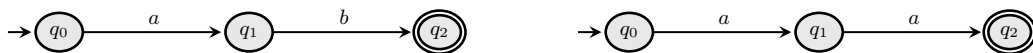
Fig. 2. Deterministic finite automata A_1 and A_2 accepting the bideterministic and finite languages L_1 = \{ab\} and L_2 = \{aa\} , respectively. In both drawings the non-accepting sink state is not shown. The longest simple path in both automata is of length 3 (including the non-accepting sink state) and the pumping constants of the languages are \text{mpe}(L_1) = 3 and \text{mpe}(L_2) = 4 .
