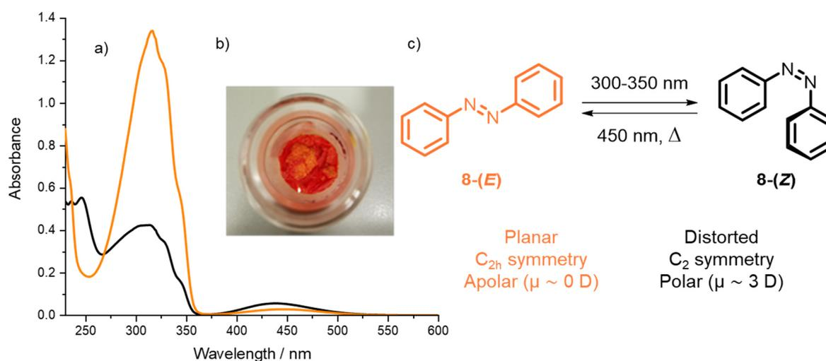
**Figure 5: a) UV-Vis spectra of unsubstituted AB 8 in *n*-decane. Red spectrum: 8-(*E*), black spectrum: 8-(*Z*). b) Solid AB 8. c) Isomerization and characteristics of unsubstituted AB 8.<sup>[6]</sup>**
