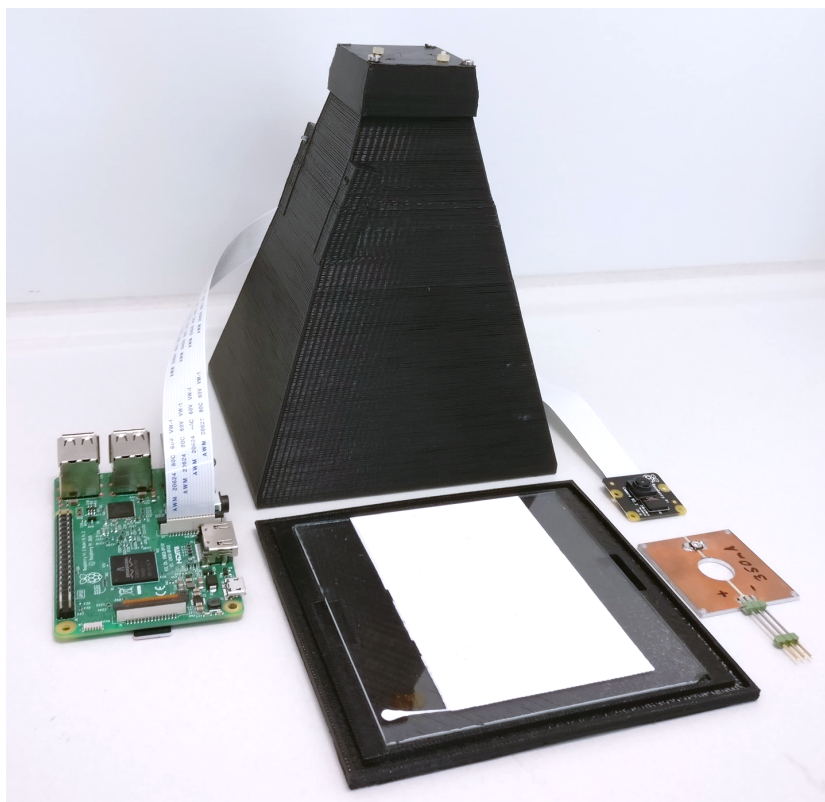
Figure S-3. 3D printed prototype for studying of the illumination at UV 254 nm, showing the baseplate carrying a self-printed layer on a 10 x 10 cm 2 glass plate and cover to be placed on baseplate.
