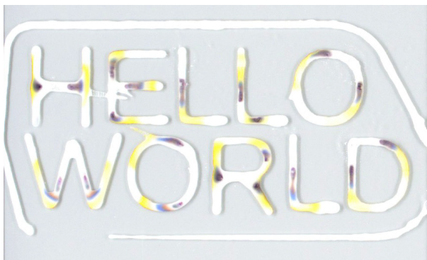
Figure S-4. 3D printing of different layer shapes and patterns: example to trigger ideas for novel planar chromatographic separations.
