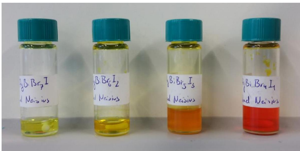
Figure S1. Pictures of the DMF solutions used for the preparation of the (\text{BA})_4\text{AgBiBr}_{8-x}\text{I}_x (with x = 1,2,3,4 ) thin films. From left to right: (\text{BA})_4\text{AgBiBr}_7\text{I} , (\text{BA})_4\text{AgBiBr}_6\text{I}_2 , (\text{BA})_4\text{AgBiBr}_5\text{I}_3 and (\text{BA})_4\text{AgBiBr}_4\text{I}_4
