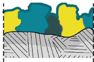
Figure 31. Representation of SEI including detailed structural and chemical information, on a particle with well-defined structure.
