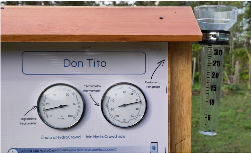
FIGURE 2 The three sensors mounted on a weather station at “Don Tito” in Honduras: a hygrometer for relative humidity, a thermometer for air temperature and a rain gauge for rainfall measurements.
