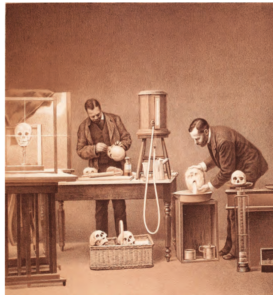
Billings, J.S.; Matthews, Washington: Ascertaining capacity of cranial cavity by means of water. Illustration in: Billings, J.S.; Matthews, Washington: "On Composite Photography as Applied to Craniology, and on Measuring the Cubic Capacity of Skulls." In: Memoirs of the National Academy of Sciences , Vol.3, part 2. Washington: Government Printing Office, 1886, 105-121.
