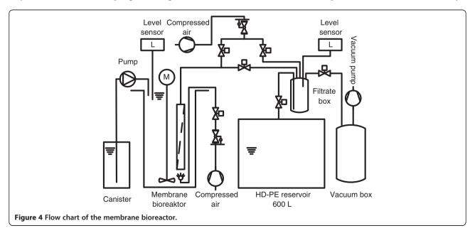
respectively), for which fresh sludge was used; the decanted water of the prior batch was reused to reduce dilution of the waste water. The biologically treated waste water was collected in a 600-L HD-PE reservoir, which was aerated during treatment, and then stored at 4°C until further use. The term *biologically treated waste water* used in this publication refers to this mixed sample.
