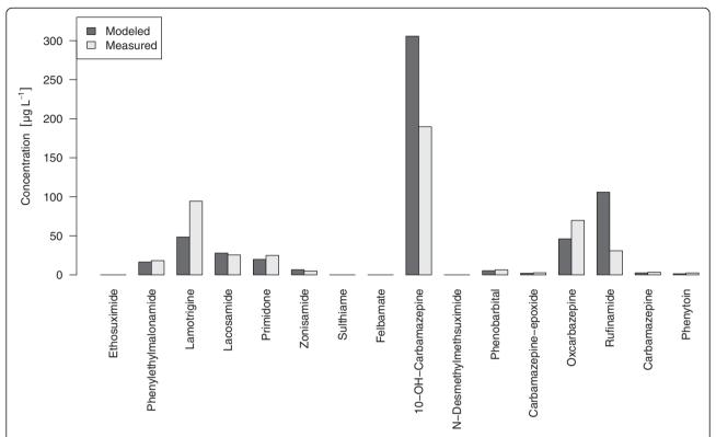
**Figure 1 Comparison of modeled and measured concentrations for biologically treated waste water.** Modeled concentrations consist of results from raw waste water samples and their fractions on the biologically treated waste water.
