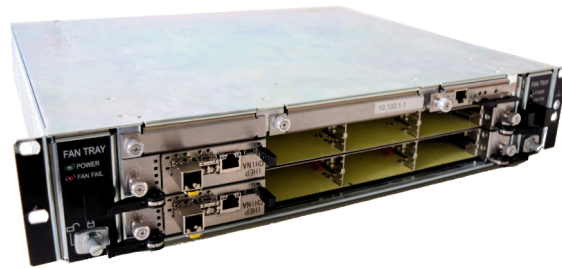
(A) ATCA shelf with two slots and two ONSEN CNCBs plugged into. Each carrier board was equipped with just one AMC. This reduced setup already enables to perform tests with Merger and Selector firmwares. The setup was used for first tests with CNCBs as well as for tests performed at DESY in 2016. a
