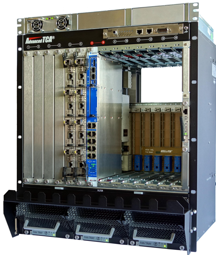
(B) ATCA shelf with two ONSEN CNCBs. This shelf was used for most tests carried out in Gießen but also for tests at DESY in 2017. Photo courtesy of T. Geßler.
