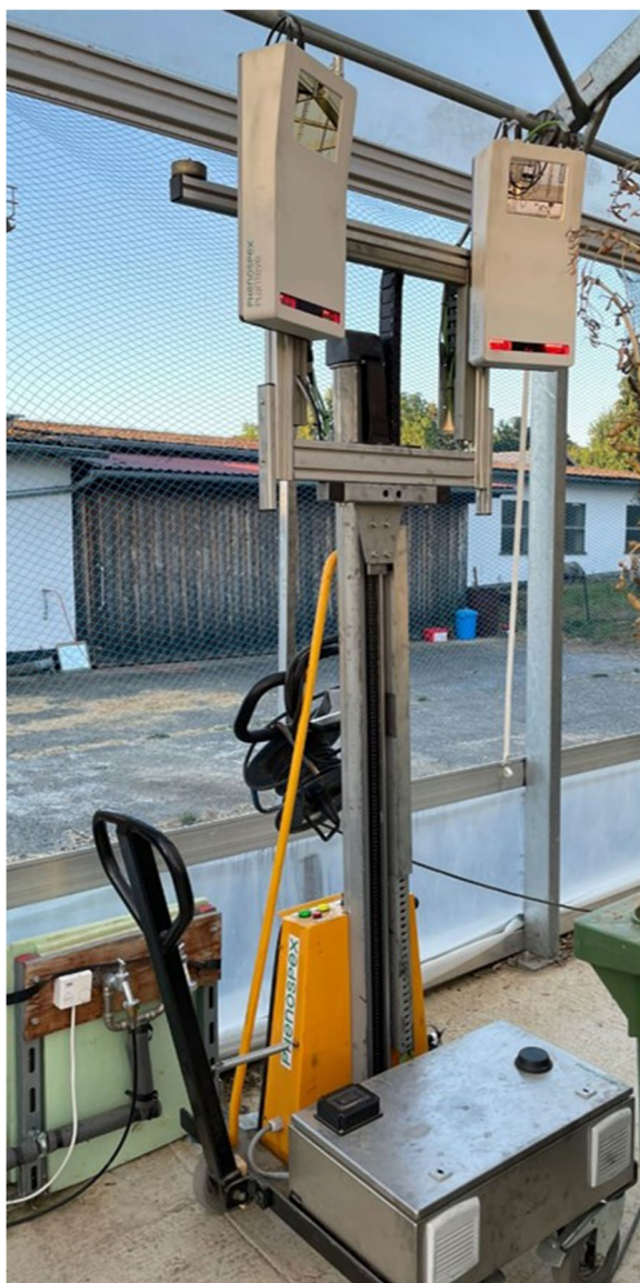
Fig. 2 Customized version of the PlantEye® 3D-Scanner used in the DroughtSpotterXXL phenotyping platform
