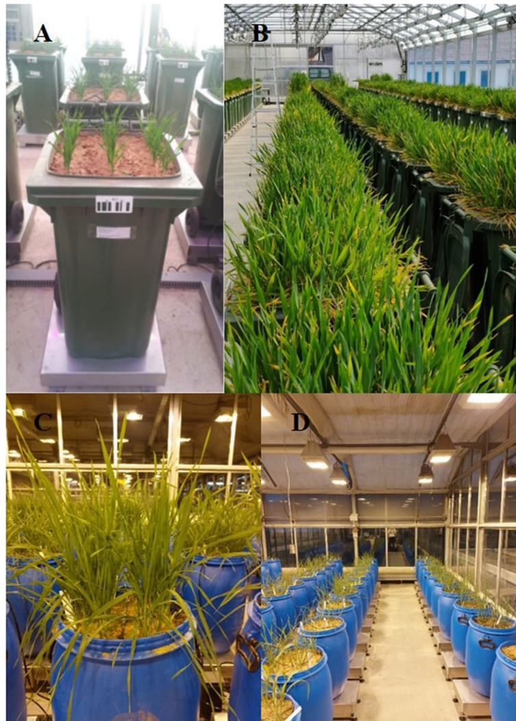
Fig. 1 General Setup of the DroughtSpotter® phenotyping platforms located at the University of Giessen (A) 90L growth container placed on weights scale in DroughtSpotterXXL with 48 wheat plants sown in three rows á 16 plants (B) Impression of the full DroughtSpotterXXL test facility (C) 60L growth container placed on weight scale in DroughtSpotterL with 16 plants (D) Impression of the full DroughtSpotterL test facility
