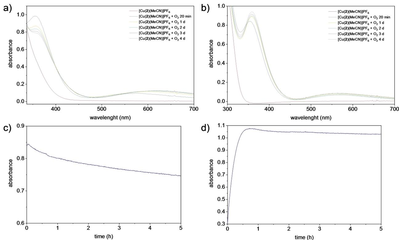
**Figure 4.** UV-vis spectra of the reaction of [Cu(**2**)(MeCN)]PF<sub>6</sub> with O<sub>2</sub> a) in acetone over 4 d and b) in DCM over 4 d; c) Time trace of the absorption at 365 nm in acetone; d) Time trace the absorption at 365 nm of the reaction in DCM.
