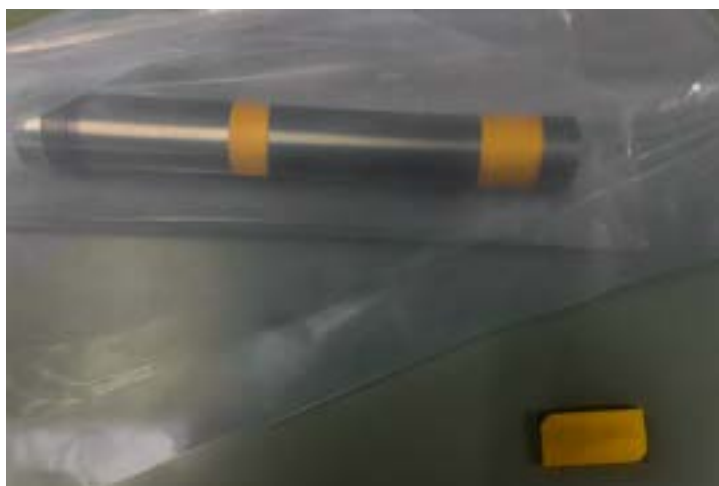
Figure 4.2: An image of the inner beryllium beam pipe with additional fragments of gold coating added (credit: Shuji Tanaka, KEK).
