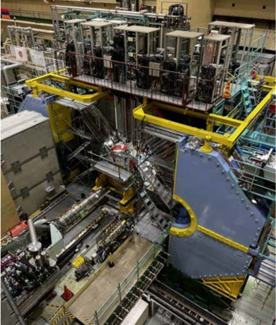
Figure A.2: Picture of the Belle II detector taken in February 2023 during the under- going LS1. The partially disassembled state reveals detector components that are usually hidden behind the detector shielding. In particular, the QCS magnet, the ARICH and the KLM are visible.
