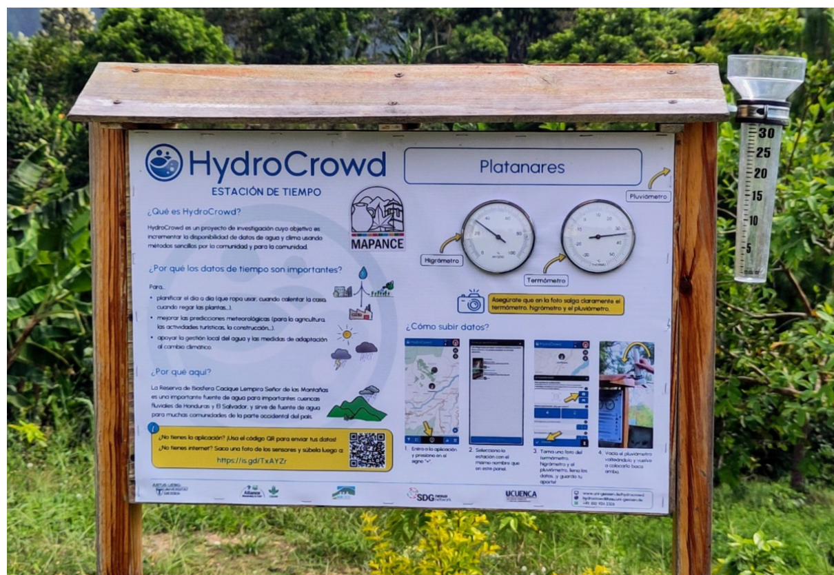
Figure 3.5: Weather station in Honduras, consisting of a wooden structure, a signpost with general information (left side) and instructions how to upload data (lower right side), and three analog sensors: a hygrometer for relative humidity, a thermometer for temperature and a rain gauge for rainfall (upper right side from left to right).
