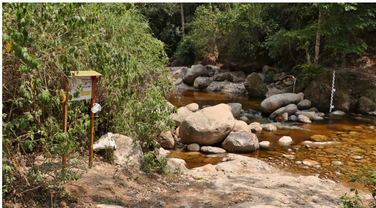
Figure 1.11: Example of a HydroCrowd water station (left) from Honduras with the corresponding water level gauges (right) mounted on a big rock in the water (own photograph from April 30, 2024).
