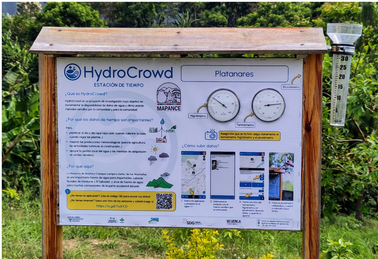
Figure 1.10: Example of a HydroCrowd weather station from Honduras with the three analog sensors: a hygrometer, a thermometer and a rain gauge (upper right side of the wooden panel from left to right; adapted from Mitze et al. (2026)).
