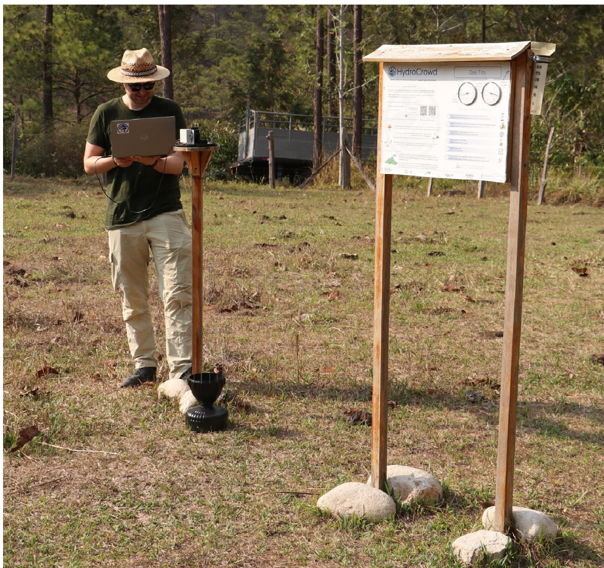
Figure 1.12: Example of a HydroCrowd weather station in Honduras with a hidden temperature/humidity sensor behind the station (right) and a tipping bucket for automated rainfall monitoring (left), which was accessed during fieldwork (photograph by Suzanne Jacobs from the June 11, 2023).
