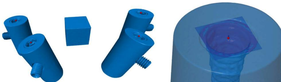
**Figure 2** X-ray computed implant-abutment interface points on the top part of the implant (red dots: IAIPs highly magnified (left); detail magnification (right)).
