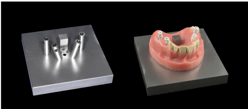
**Figure 1** Implant master model (IMM) with four steel tubes (angulation 0° and 15°), reference cube (left) and final setup with fixed scan bodies (nt-trading, right).
