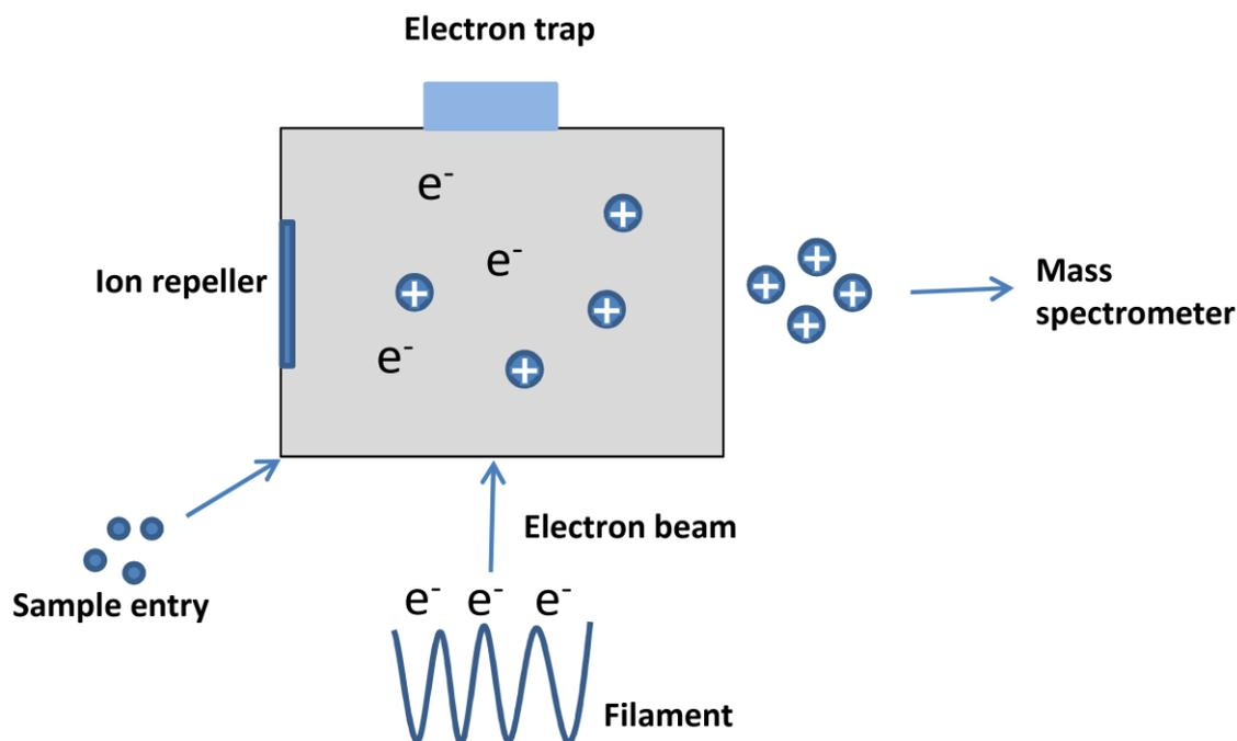
Figure 12. Diagram of an EI ion source. High-energy electrons are obtained from a heated filament and interact with the analytes to produce positive ions.
