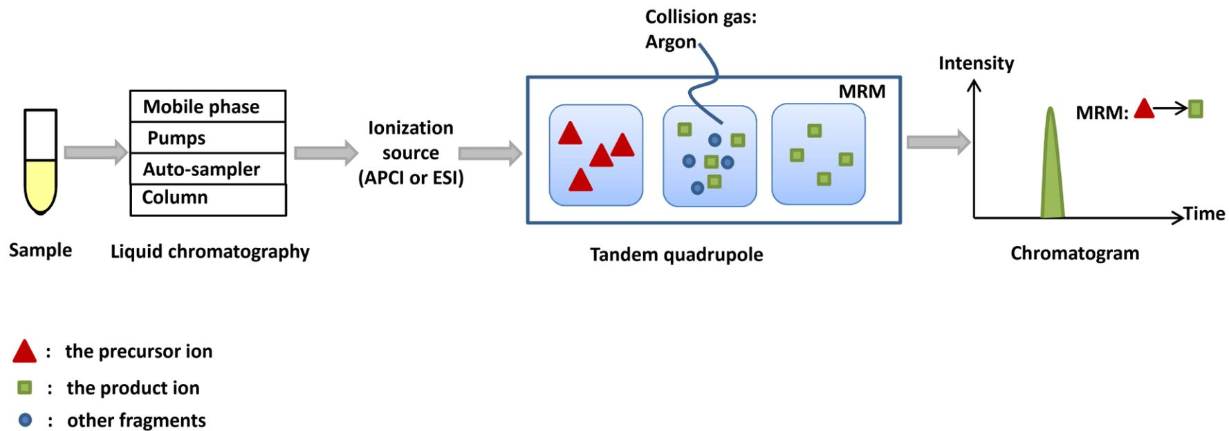
Figure 11. Representation of a typical LC-MS/MS operating in MRM mode. Samples are separated by liquid chromatography, ionized in the ion source, and enter the tandem quadrupole. Q1 selects the precursor ions, Q2 breaks the precursor ions into fragments and Q3 selects the product ions.
