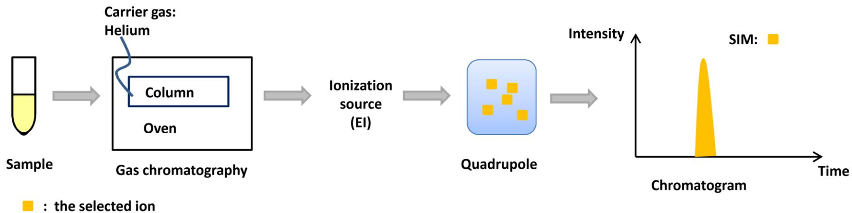
Figure 13. Representation of GC-MS analysis in SIM mode. Samples are separated by gas chromatography, ionized in the ion source, and enter the quadrupole. The selected ions are monitored and detected.
