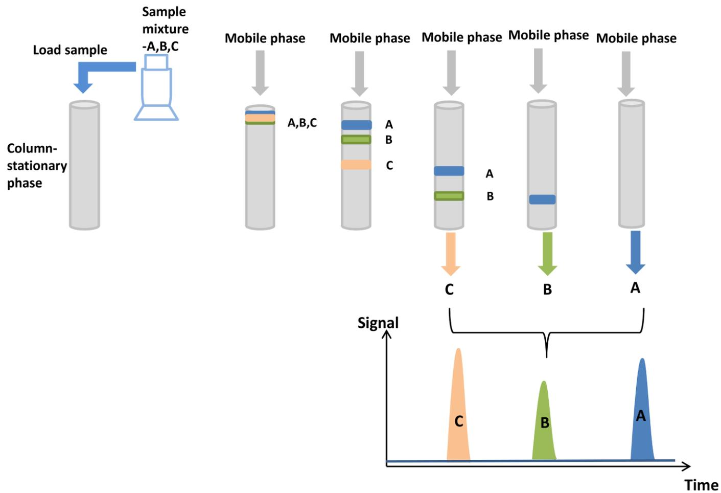
Figure 8. Schematic diagram of chromatography. Sample mixture containing A, B and C are loaded on the column and eluted by mobile phase according to their partition coefficient.
