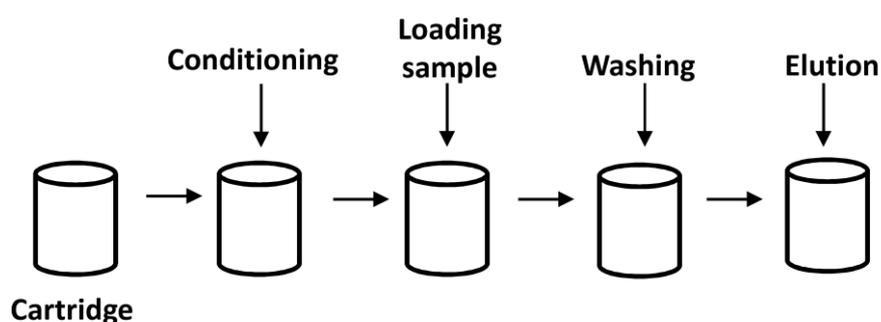
Figure 14. General steps for solid phase extraction
