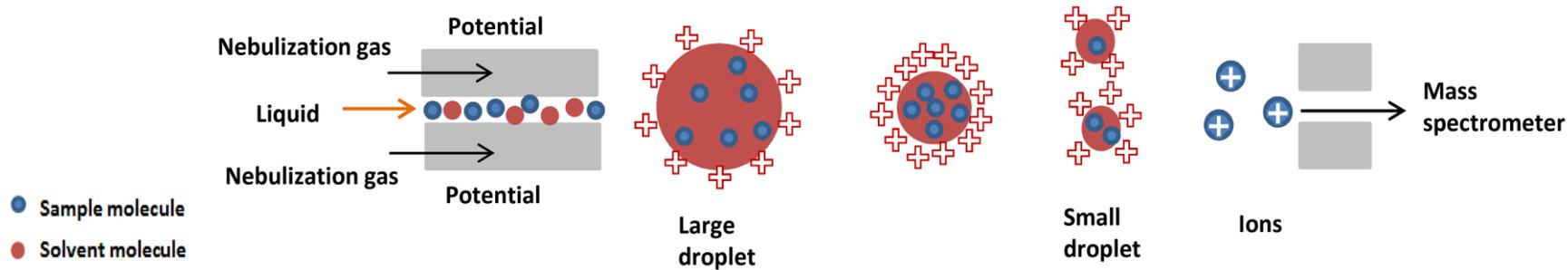
Figure 9a. Schematic representation of ESI ion source.
