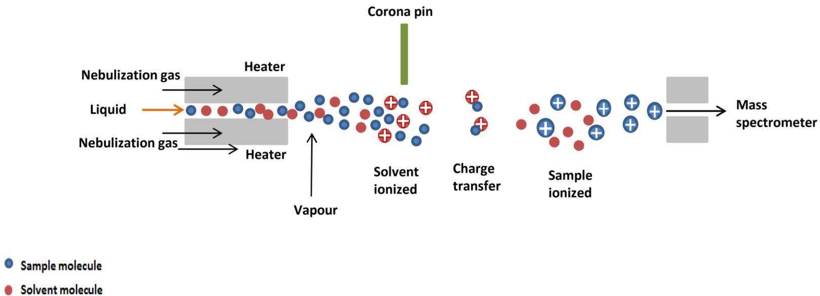
Figure 9b. Schematic representation of APCI ion source.
