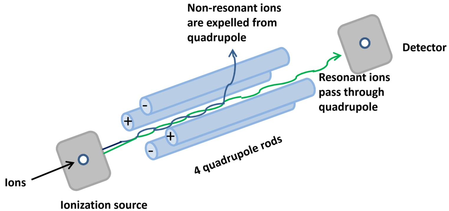
Figure 10. Schematic display of a quadrupole mass analyzer.
