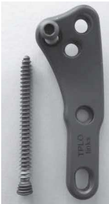
Fig. 1 Custom made left titanium tibial plateau levelling osteotomy implant.
