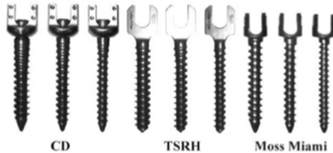
Fig. 1. Three different pedicle screws tested in this study. Each had three types—I, II, and III—corresponding to different outer diameters.
