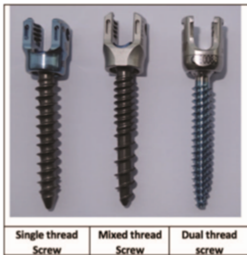
Figure 1. Pedicle screw design details.
