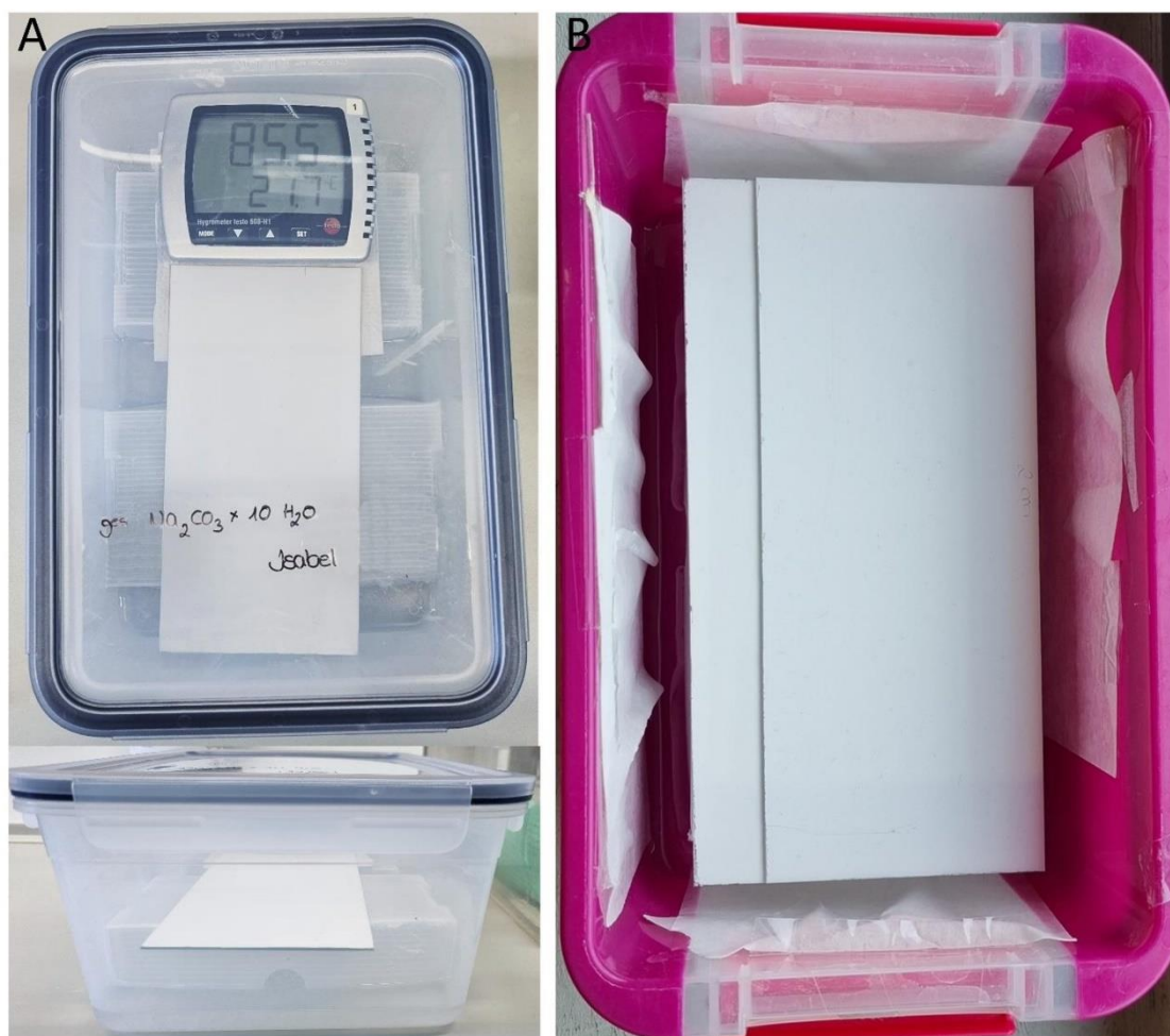
Fig. S1. Standardization of the plate humidity: (A) Plastic box for pre-conditioning filled with 200 mL saturated sodium carbonate and (B) a smaller plastic box for incubation at 37 °C lined with wet filter paper and filled with 70 mL water.
