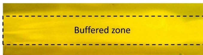
Figure S6: Influence of the phosphate-citrate buffer pH 12 on HPTLC RP-18 W plates after the derivatization with rhodamine 6G reagent, detected at FLD 366 nm.
