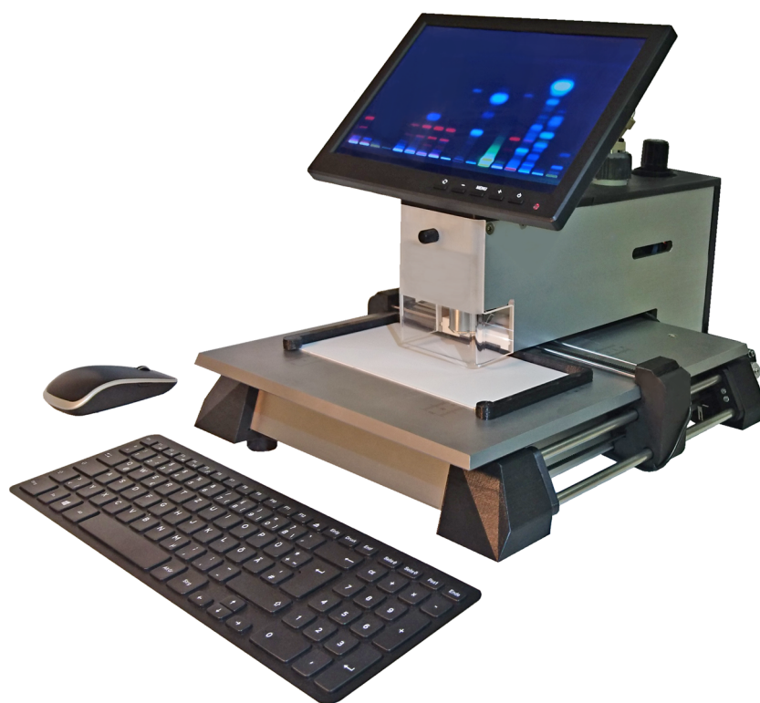
FIGURE 4 The autoTLC-MS Interface, a 3D-printed add-on package for automated plate positioning (mounted on the base part of the TLC-MS Interface 2) with integrated automatic 2/6-port valve and four magnetic valves for pneumatic functions. The IPS display and the communication port were mounted on the top and on the rear side of the interface and can be connected to the advanced NUC system (not displayed) [Color figure can be viewed at wileyonlinelibrary.com ]
