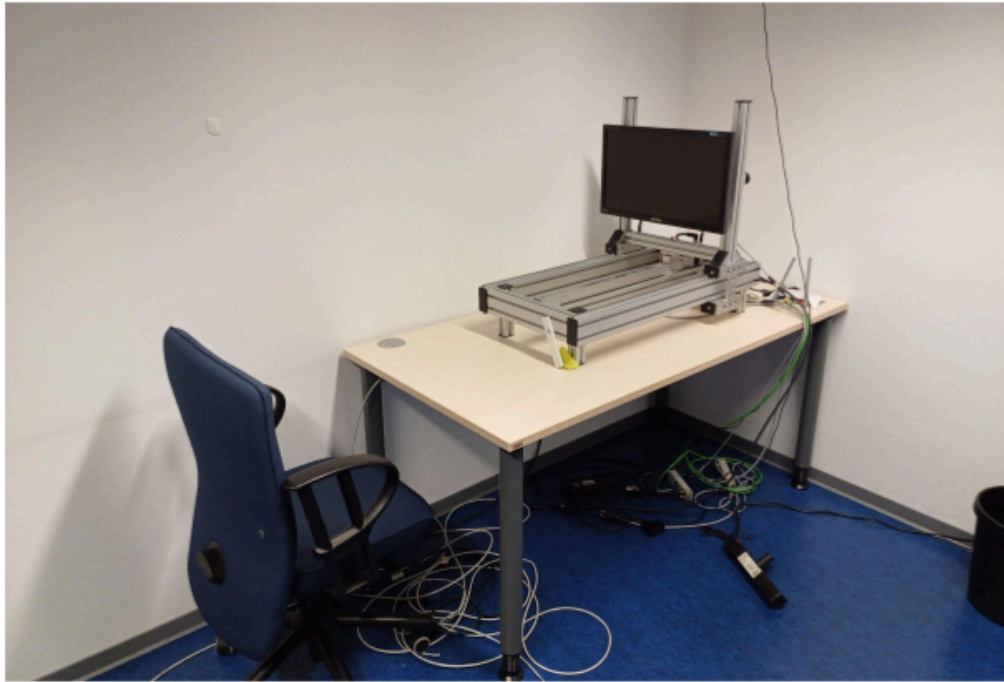
Figure 29: The moving monitor. A 22 inch monitor attached to a spindle axis, allowing the screen to be moved back and forth over a range of 60cm.
