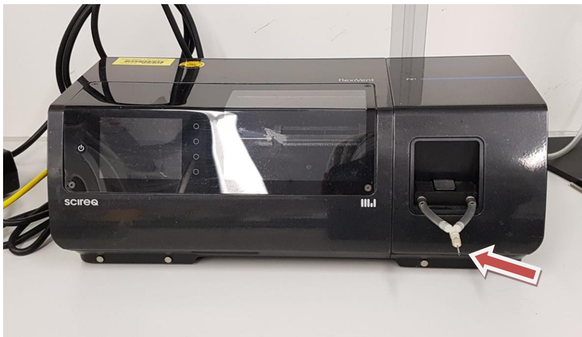
Figure 5: ScireQ Oszillationplethysmograph (Scireq, FlexiVent) for lung function measurement
