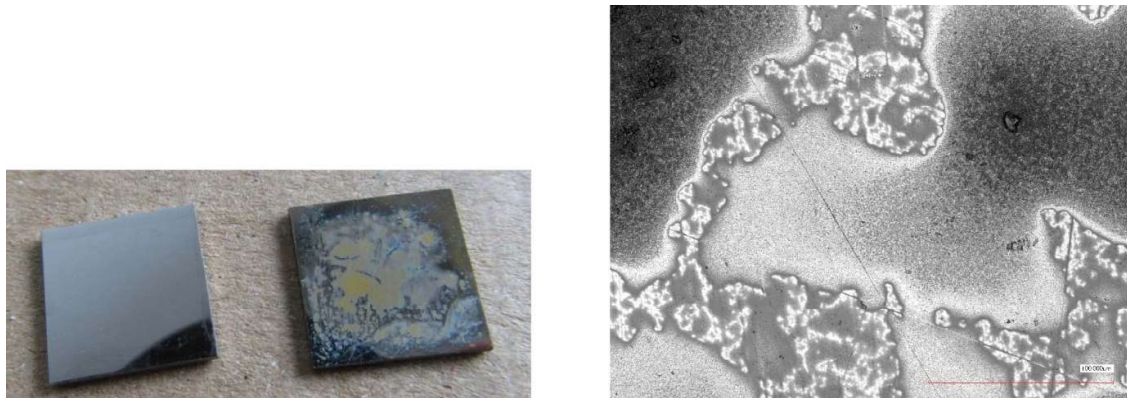
(a) S/S macroscopic; left is reference sample, right is plasma-treated (b) Laser microscopic S/S image (plasma-treated)
