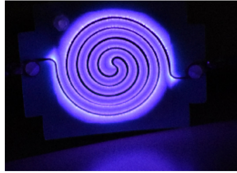
FIGURE 2.7: Picture of the plasma light at the grounded electrode of the sputter-coated DBD prototype. A homogeneous plasma discharge is visible. [44]
