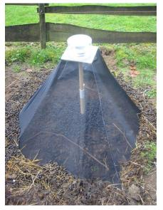
Fig. 11. BG-Sentinel<sup>TM</sup> UV light midge trap. Insects are attracted by black light and sucked into a catch beaker by fan (Mehlhorn *et al.* 2009a).
