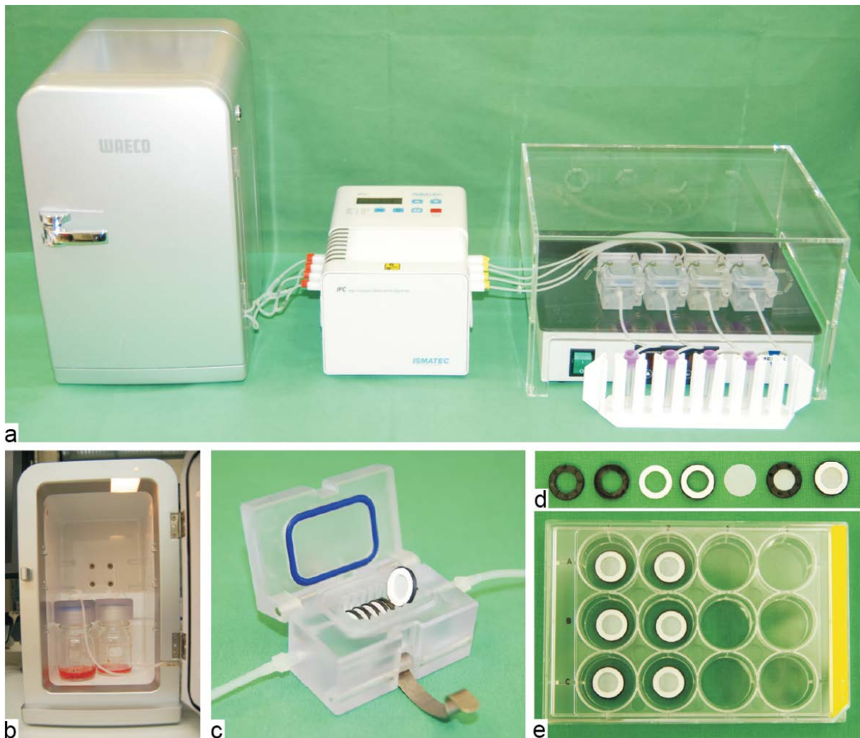
Figure 3-2 The Tissue Factory™ (a) complete perfusion apparatus (b) medium cooler with supply bottles (c) perfusion chamber with cell carriers (d) detailed aspects of the tissue carriers and their assembly (e) preculture of tissue carriers in 12-well plates.
