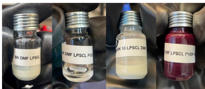
Figure 36: Left: suspension of LPSCI in DMF, no discoloration. Center-left: solution of PVDF in DMF, no discoloration. Center right: dispersion of LPSCI in a solution of PEO in DMF (for reference), no discoloration. Right: dispersion of LPSCI in a solution of PVDF in DMF, discoloration and formation of a thick slime.
