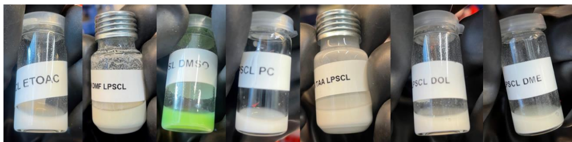
Figure 35: LPSCI powder submerged in ethyl acetate, DMF, DMSO, propylene carbonate, 2-methyl-2-butanol, DOL, and DME (from left to right). While contact to DMSO instantly led to discoloration, all the other combinations did not change their optical appearance over several days.
