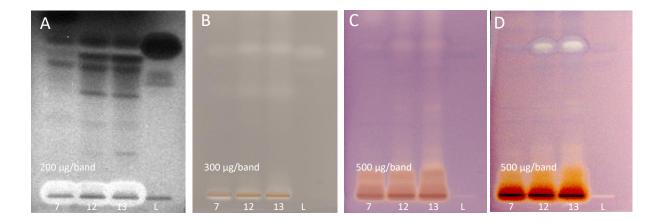
**Figure S11** Co-chromatography of cinnamon extract IDs 7, 12 and 13 (200–500 µg/band depending on the assay) along with linoleic acid (L; 2.5 µg/band) on HPTLC plates silica gel 60  $F_{254}$  with toluene – ethyl acetate – methanol 6:5:3 (V/V/V) detected via (**A**) the bioluminescent *Aliivibrio fischeri* bioassay, and at white light illumination, (**B**) the tyrosinase, (**C**)  $\alpha$ -glucosidase and (**D**) AChE inhibition assays.
