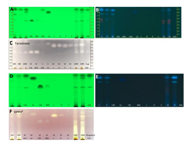
**Figure S9** Co-chromatography of cinnamon extract IDs 1, 7, 8, 12 and 13 along with cinnamaldehyde (CAD), coumarin (Co), cinnamic acid (CIN), benzoic acid (BEN), linoleic acid (L), oleic acid (O), stearic acid (S) on HPTLC plates silica gel 60  $F_{254}$  with toluene - ethyl acetate - methanol 6:5:3 (V/V/V), detected at (A/D) UV 254 nm, (B/E) FLD 366 nm and (C/F) white light illumination for tyrosinase inhibition and DPPH $^{\bullet}$  assays.
