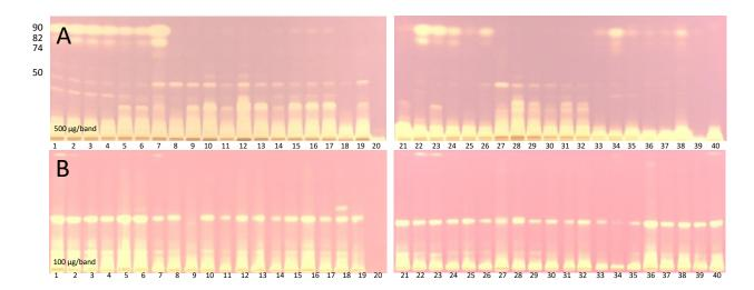
**Figure S8** DPPH• radical scavenger screening of cinnamon extract IDs 1-40 (500  $\mu$ g/band for A and 100  $\mu$ g/band for B) on HPTLC plates silica gel 60 F<sub>254</sub> with (**A**) toluene – ethyl acetate – methanol 6:5:3 *versus* a mobile phases of higher elution power with (**B**) ethyl acetate – toluene – formic acid – water 16:4:3:2, both V/V/V.
