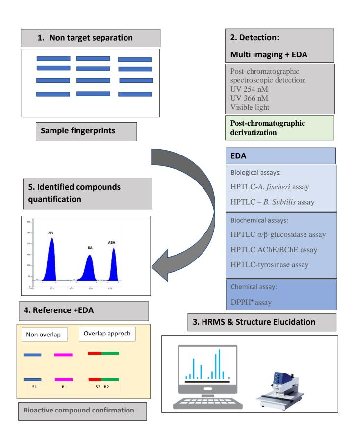
**Figure 6.** Schematic diagram describes HPTLC-UV/Vis/FLD-EDA-HESI-HRMS analytical platform which was designed to identification of bioactive compounds in *Abelmoschus moschatus* and *Cinnamomum zeylanicum*.
