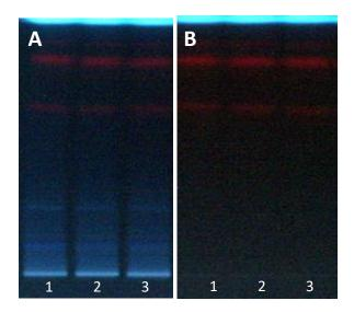
**Figure S2** Extraction solvent selection: HPTLC chromatograms at FLD 366 nm of cinnamon IDs 1-3 (1  $\mu$ L, 100 mg/mL, 100  $\mu$ g/band) (**A**) extracted with methanol – water and (**B**) ethyl acetate – *n*-hexane, for both 4:1, *V/V*, on HPTLC plate silica gel 60 F<sub>254</sub> with ethyl acetate – methanol – water 17:2:1 (*V/V/V*).
