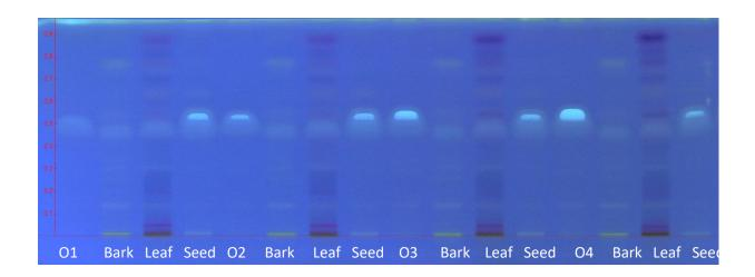
**Figure S7** Comparison of oleic acid content of *Abelmoschus moschatus* in the different plant parts: HPTLC chromatogram with oleic acid standard levels (O1-O4; 3, 6, 9 and 12 μL/band; 1.35 mg/mL) and bark (ID 2, 20 μL, 1340 μg/band), leaf (ID 9, 12 μL, 1200 μg/band) and seed (ID 10, 2 μL, 200 μg/band) extracts applied four-fold on HPTLC plate silica gel 60  $F_{254}$  developed with toluene - ethyl acetate 7:3 (V/V) up to 65 mm, detected and documented as before
