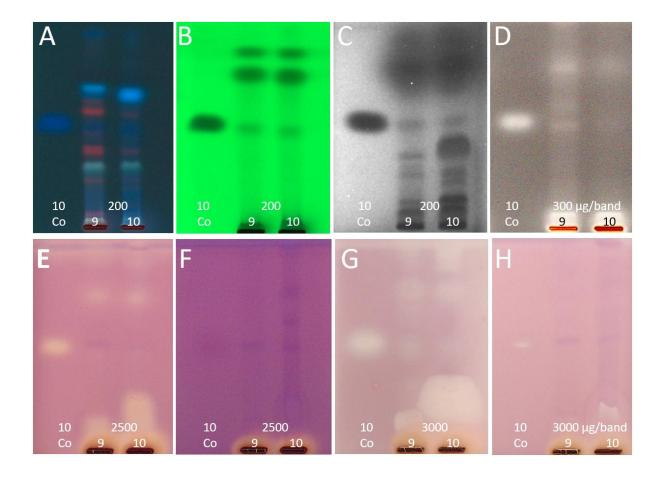
**Figure S14** Bioactivity of coumarin (Co, 10 μg/band) and cinnamon extract IDs 9 and 10 (200–3000 μg/band depending on the assay) on HPTLC plates silica gel 60 with n-hexane – ethyl acetate – ammonia 3.8:1.3:0.05, V/V/V, detected at (**A**) FLD 366 nm, (**B**) UV 254 nm, (**C**) via bioluminescent A. fischeri bioassay, (**D**) tyrosinase, (**E**)  $\alpha$ -glucosidase, (**F**)  $\beta$ -glucosidase, (**G**) AChE and (**H**) BChE inhibition assays.
