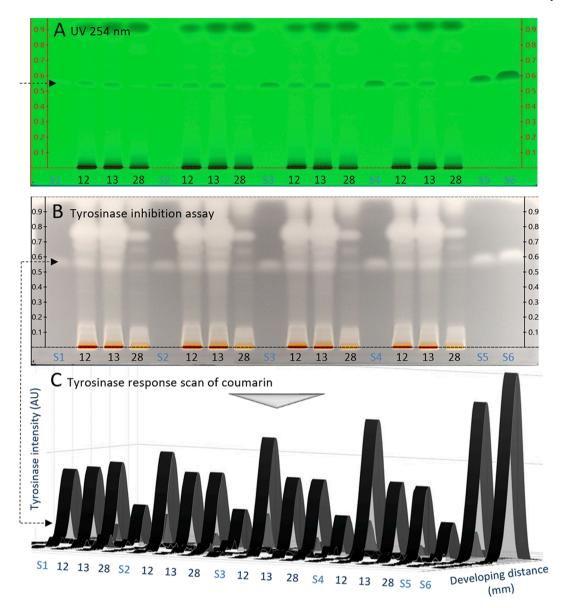
Fig. 4. Enzymatic quantification of the cinnamic acid via its tyrosinase inhibition response in cinnamon extract IDs 12, 13 and 28 (300 μg/band each) via cinnamic acid (S1–S6, 0.25–2.0 μg/band): (A) pre–assay UV 254 nm chromatogram, (B) tyrosinase inhibition autogram and (C) respective inverse scan densitograms at 579 nm.
