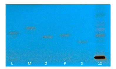
**Figure S12** Co-chromatography of linoleic acid (L), myristic acid (M), oleic acid (O), palmitic acid (P), stearic acid (S; 25  $\mu$ L, 0.5 mg/mL, 12.5  $\mu$ g/band each) and cinnamon t-butyl methyl ether extract ID 12 (25  $\mu$ L, 100 mg/mL, 2500  $\mu$ g/band) on HPTLC plate silica gel RP 8 F<sub>254S</sub> with methanol – water – formic acid 9:1:0.1 (V/V/V) up to 70 mm, detected at 366 nm using the primuline reagent.
