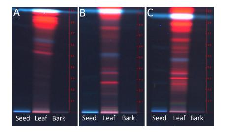
**Figure S3** Mobile phase optimization study (all V/V): HPTLC chromatograms of *Abelmoschus moschatus* ID 1 seed, leaf (each 250 µg/band) and bark (80 µg/band), applied on HPTLC silica gel 60 F<sub>254</sub> plates and developed with (**A**) n-hexane – acetone - water 7:7:0.2, (**B**) toluene - ethyl acetate - methanol 6:5:2 and (**C**) n-hexane - toluene - ethyl acetate - methanol - water 2:5:5:2:0.2, all up to 65 mm and documented at FLD 366 nm
