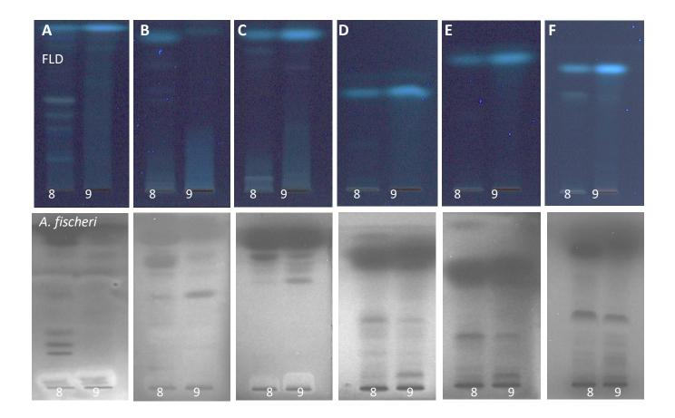
**Figure S4** Extended mobile phase selection with regard to effects: HPTLC chromatograms of cinnamon extract IDs 8 and 9 (each 2  $\mu$ L, 100 mg/mL, 200  $\mu$ g/band) on HPTLC silica gel 60 plates with (**A–E**) mobile phases as in Figure S3 and (**F**) ethyl acetate – toluene 1:1, all up to 70 mm, documented at FLD 366 nm and after the bioluminescent *Aliivibrio fischeri* bioassay (greyscale image).
