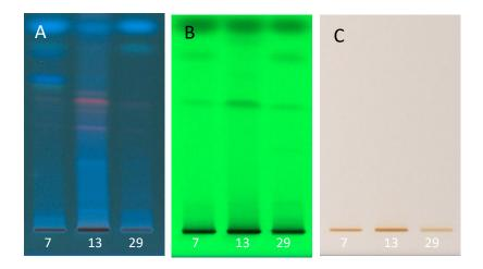
Figure S5 Selected mobile phase: HPTLC chromatograms of cinnamon extract IDs 7, 13 and 29 (each 2  $\mu$ L, 100 mg/mL, 200  $\mu$ g/band) on HPTLC plates silica gel 60 F<sub>254</sub> with toluene – ethyl acetate – methanol 6:5:3 (V/V/V; as in Figure S3/4 B) up to 70 mm, documented at (**A**) FLD 366 nm, (**B**) UV 254 nm and (**C**) white light illumination.
