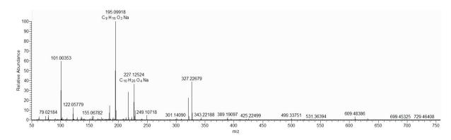
**Figure S5** HPTLC-HESI<sup>+</sup>-HRMS spectra recorded of the bioactive multi-potent zone in the seed extract ID 10 in the positive ionization mode showing the respective sodium adduct of the oxidized degradation products 8-oxo-decanoic acid at m/z 195.0991 [ODP1+Na]<sup>+</sup> (base peak) and dihydroxydecanoic acid at m/z 227.1252 [ODP2+Na]<sup>+</sup>
