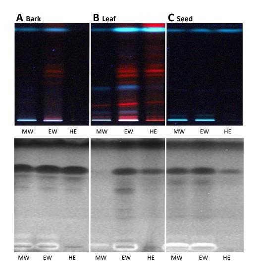
Figure S2 Extraction solvent selection: HPTLC chromatograms of *Abelmoschus moschatus* ID 1 (A) bark (80 µg/band), (B) leaf and (C) seed (250 µg/band) extracted with methanol – water (MW), ethanol – water (EW) and n-hexane – ethyl acetate (HE), all 4:1 V/V, separated on HPTLC plate silica gel 60 F<sub>254</sub> with toluene – ethyl acetate – methanol 6:5:2 (V/V/V) and documented at FLD 366 nm and after the *Aliivibrio fischeri* bioassay (greyscale image of bioluminescence)
