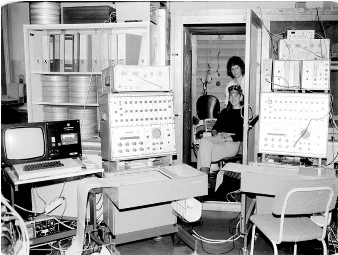
Figure 1: EEG laboratory of the Institute of Pathological Physiology Jena (1987) with the Faraday cage, two coupled 8-channel EEG devices for 16-channel recordings and the computer for data digitalization (left).
