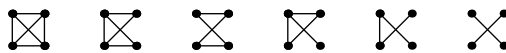
Fig. 3. All possible subgraphs that are unit squares with two diagonals up to mirroring and rotation, that can occur in a undirected grid graph with diagonals. All these subgraphs, except the last one (X-crossing), can be replaced by a unit square giving a reachability equivalent undirected graph.
