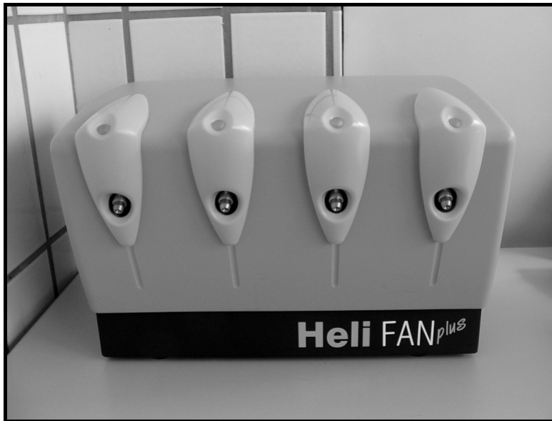
Figure 8a: ^{13}\text{CO}_2 measuring device HeliFANplus ® (Fischer Analysen GmbH, Leipzig; Germany) based on non-dispersive infrared spectroscopy.
