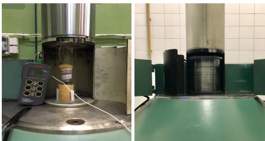
Figure 2. Examples of samples placed in the center of the chamber (in small cups, left, of in petri dishes, right). These are surrounded by a 4mm thick PMMA tube, which provides adequate build-up material. The temperature is taken before and after exposure. The temperature information is important for the dosimetry
