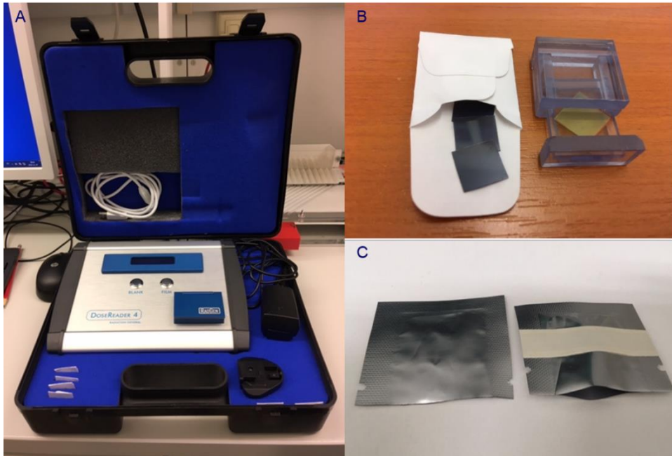
Figure 7. Gafchromic dosimetry system. A) the optical density film reader, B) paper envelope containing 3 exposed films (left), and a plastic dosimeter holder containing 1 unexposed film, and C) aluminium pouches that can be heat sealed, with an adhesive strip for sticking the envelope onto a container.
