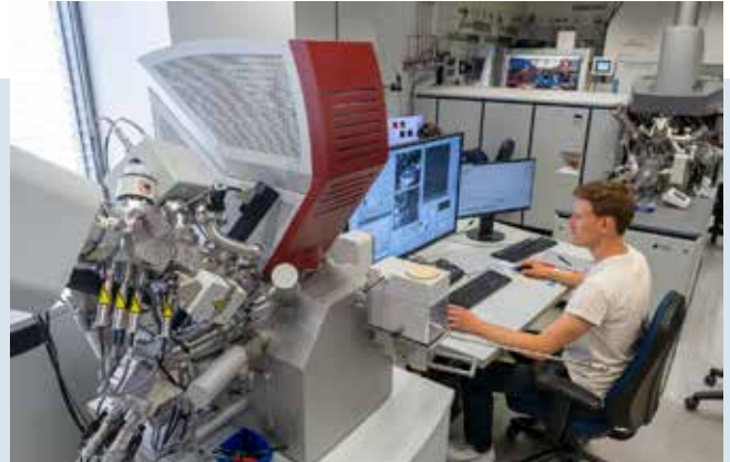
Figure 4. Battery research with large-scale equipment: Examining a cross-section through a battery sample in a focused ion beam scanning electron microscope.
