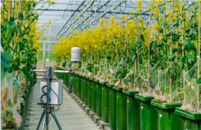
Figure 3. The DroughtSpotterXXL system is unique in the world. It automatically records plant responses to drought stress at five-minute intervals throughout the year.
