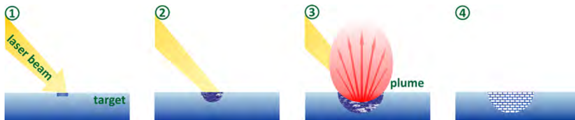
Fig. 2.14.: Schematic sketch of the laser/target interaction during the PLD process: 1) absorbance of the laser light by the solid target surface; 2) local melting of the surface; 3) evaporation of the target material in a plume; 4) resolidification of the target material after end of the laser pulse. Modified and redrawn from [106,107]
