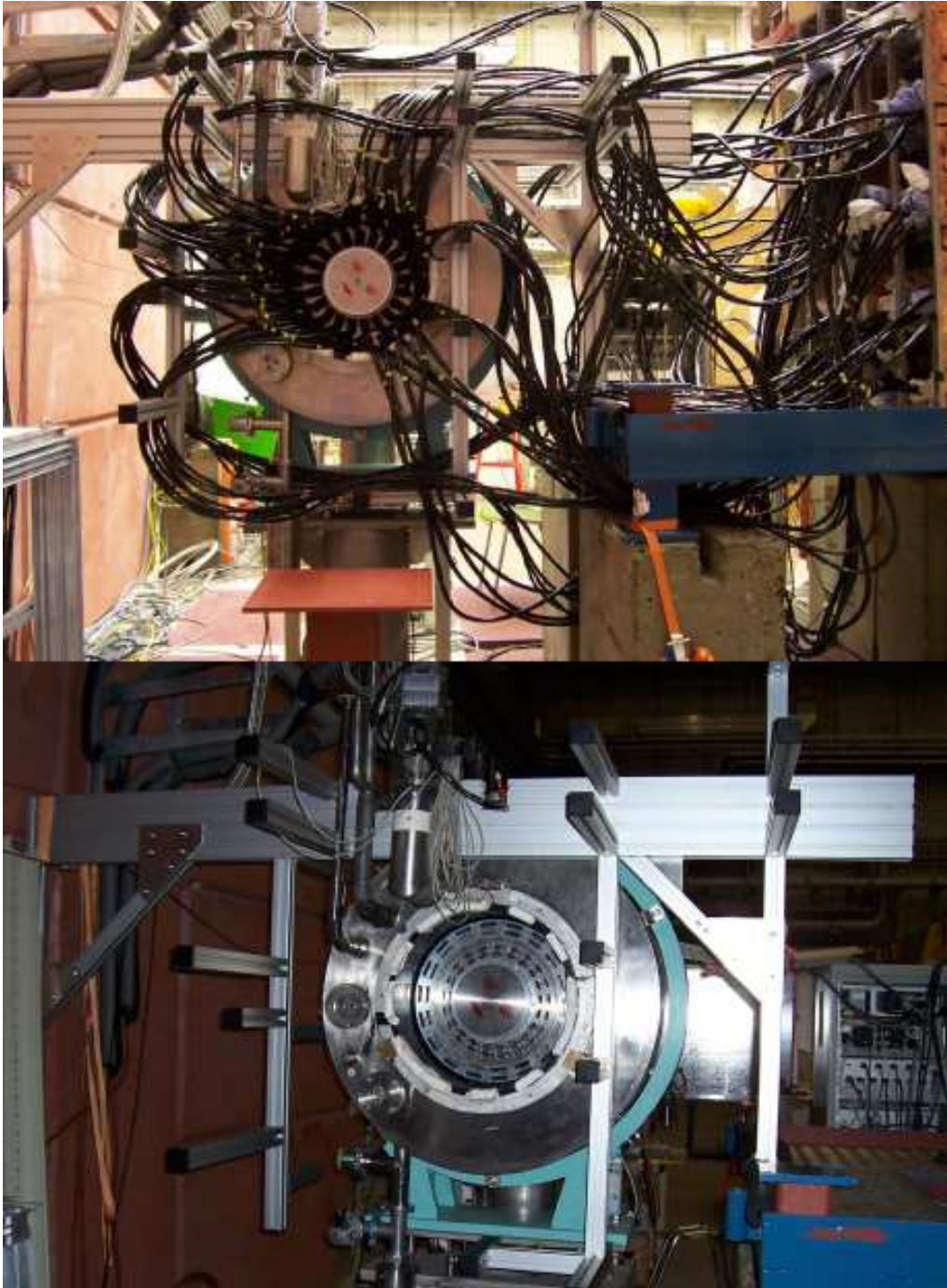
Figure 5.16: Photos of the holding structure profile installed in front of the Recoil detector at the East Hall during the cosmic test experiment, with the light guide on top and without the light guide on bottom.
