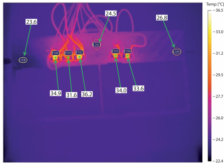
Figure 5.24: Short stave cooling test: temperature of the five resistors on the back side, as well as of some points on the stave; the water flows from left to right. The highest temperatures are measured on the first and third resistors from left, which are placed on the non-conductive part of the FPC. The second resistor from left is glued on the copper heat sink on the FPC and has the lowest temperature among all resistors. The two dummy chips on the right are glued directly on the carbon fiber and their temperature is between those of the other resistors. The rightmost point on the stave is measured directly on the carbon fiber; the two points on the left are measured on the FPC and feature lower temperatures, since they are partially shielded from the heat dissipated in the carbon foam block underneath. The environment has a temperature of 24°C; all other temperatures are also in °C.
