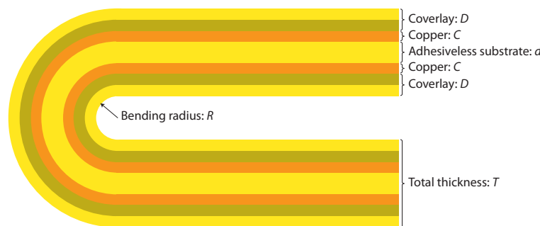
Figure 5.11: Minimum bending ratio for a double-sided flexible circuit with coverlay: definition of the layers.
