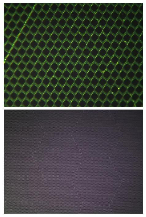
**Figure 3.14:** Microscope images of an MCP. The top picture shows a close up of individual pores with a diameter of  $10 \,\mu\text{m}$  and a hole-to-hole distance of  $12 \,\mu\text{m}$ . The *OAR* for this geometry is about 63%. The bottom picture shows a larger scale of the plate. One can see that the macroscopic MCP consists of multiple hexagonal portions. Both pictures are a courtesy of PHOTONIS.
