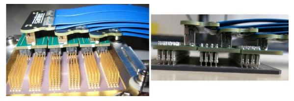
Figure 5.26: Left: 3 of 6 transmission assemblies have been connected to the Hamamatsu MCP-PMT prototype. Right: One fully equipped pin grid array of a Photonis MCP-PMT.
