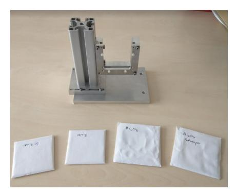
Figure 5.20: Holding structure and four packaged entrance window samples (fused silica and sapphire) for the test of radiation induced loss of transparency.
