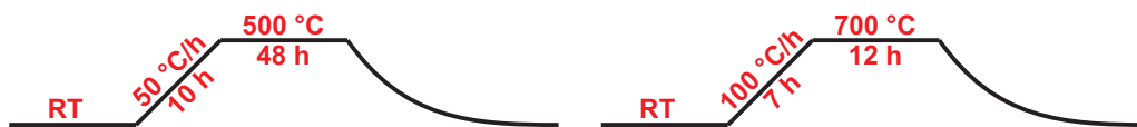
Figure 5.18: Schematic drawing for the two step annealing route of all fused silica dielectric plates starting at room temperature (RT).
