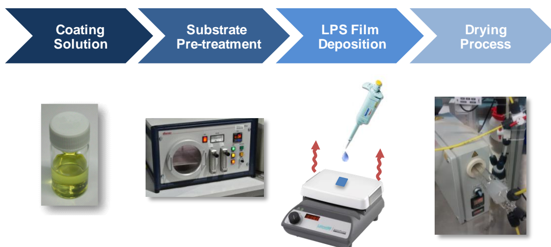
Figure 4-7: Schematic overview of the film formation process.
