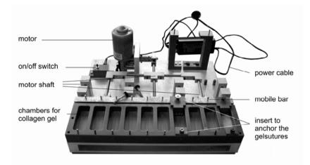
Fig. 8: Bioreactor with 10 chambers. In each chamber a collagen I gel containing ASCs was sutured, covered with medium and stretched periodically.
