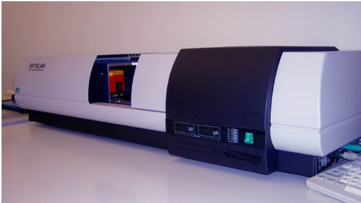
Abb. 4 SkyScan-1072 High-resolution desk-top micro-CT system
