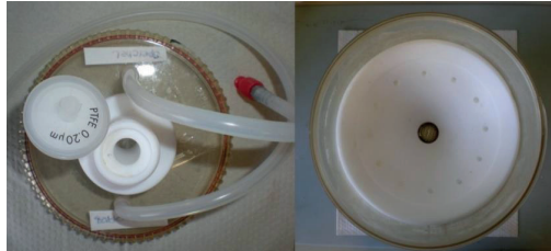
Figure 9: The screwable cap (left) and the Teflon base (right) of the reaction chamber. Chewing simulator plates with waxed specimens are placed in the 12 holes of the Teflon base. The central opening holds the pH-electrode.
