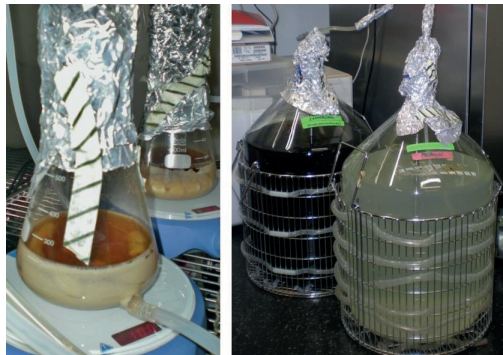
Figure 10: Containers of the caries model. Reservoir-containers with S. mutans , placed on magnetic stirrers during a double caries model (left). Note the biofilm accumulation at the inner walls of the flask after a few days of operation and the white fine-pore stones, which are visible through the bacterial solution. Artificial saliva (clear) and nutrition medium (dark) 20 l glass bottles are placed outside the incubator due to limited space (right).
