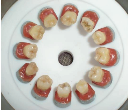
Figure 2: Placement of 12 specimens on chewing simulator plates in the reaction chamber of the caries model.
