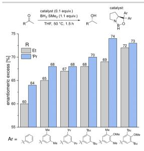
Figure 23. CBS reductions of butanone (grey) and 3-methyl-2-butanone (blue) employing modified catalysts of growing size.<sup>[4b]</sup>
