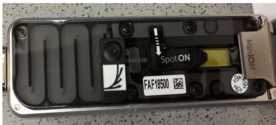
Figure 9. MiniOn portable, real-time device for sequencing (Nanopore Technologies), used for long-reads sequencing of the collected samples.
